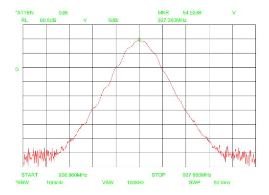
This is the highest frequency handled by the equipment under test, and is being used by the base. The frequency correspond to the last channel the equipment is using and the frequency carrier is of 927.36 MHz.
