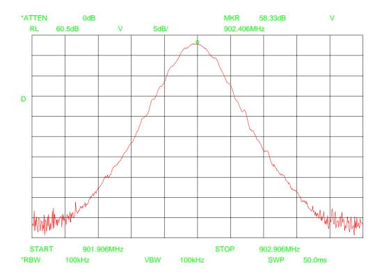
This is the lowest frequency handled by the equipment under test, and is being used by the handset. The frequency correspond to the first channel the equipment is using and the frequency carrier is of 902.406 MHz.
