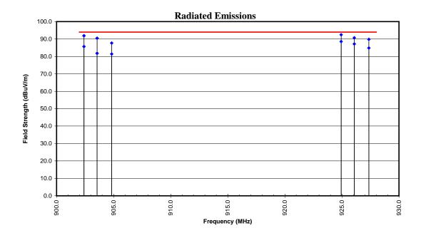
The measured data in the table above was taken using a Polarad (R&S) test receiver utilizing a Quasipeak detector.
