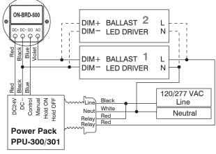
NOTE: Each PPU-300/301 power pack can supply power for up to ? ON-BRD-500 sensors. When more sensors are connected, multiple power packs may be required.
