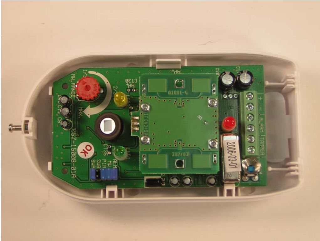
DP250 PCB top view with transmitter module installed
