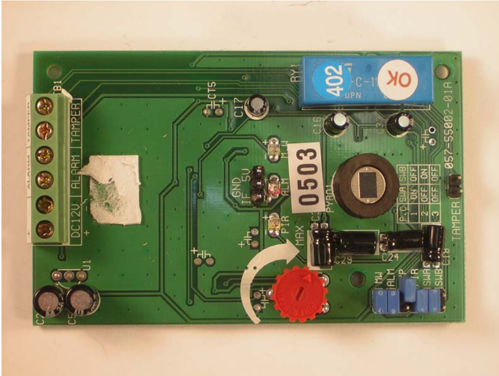
DP550P PCB top view with transmitter module removed
