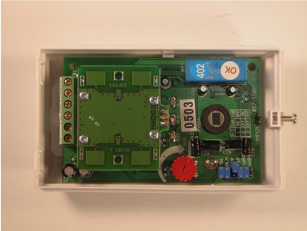
DP550P PCB top view with transmitter module installed
