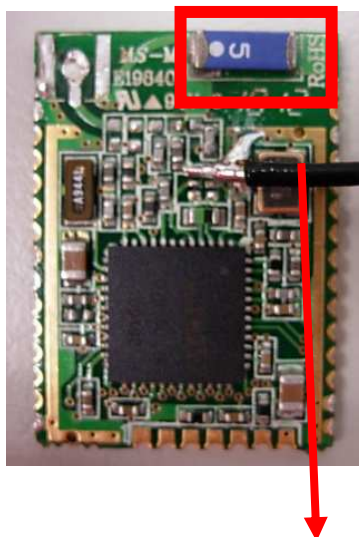
5.3*2.0 mm T5 Ceramic Chip Antenna
