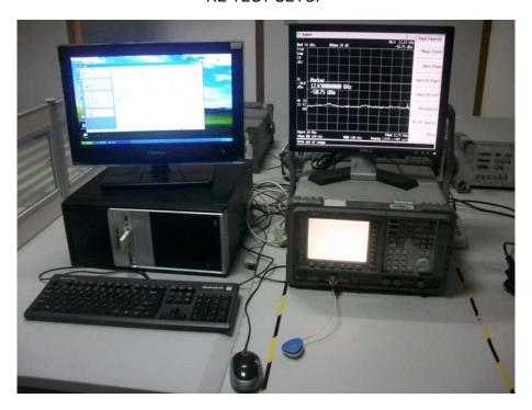
SPURIOUS EMISSION TEST SETUP
