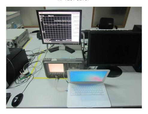
RADIATED EMISSION TEST SETUP
