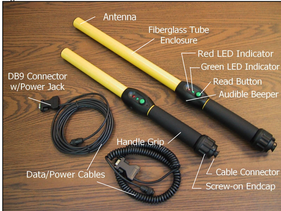
Figure 1 - Stick Reader Features and User Interface
