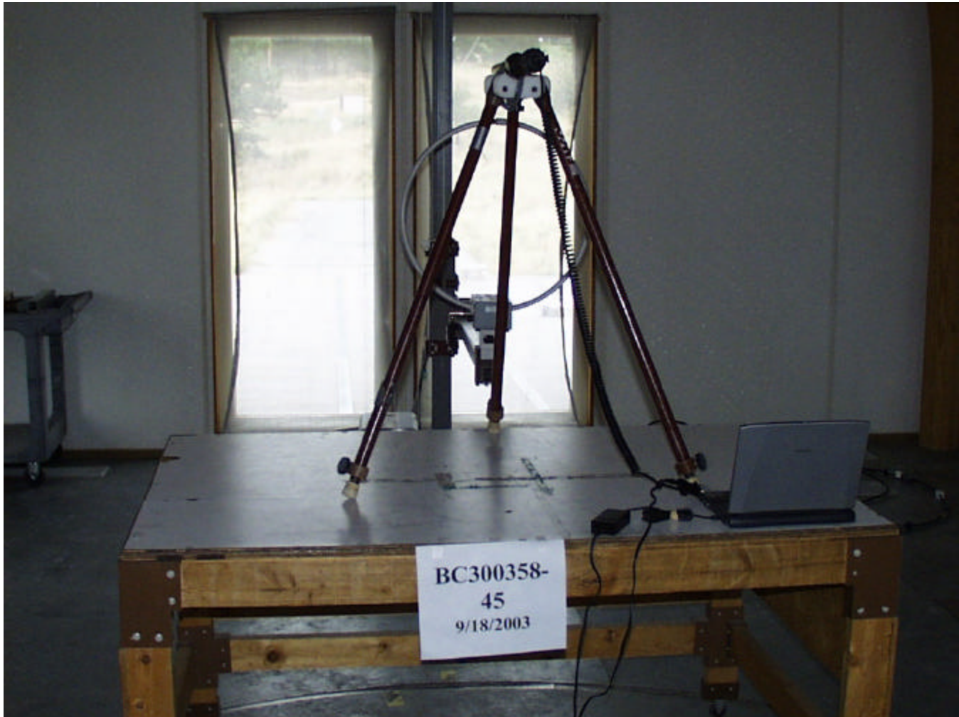
Test-setup photo(s): Intentional Radiated Emissions (60cm Device)
