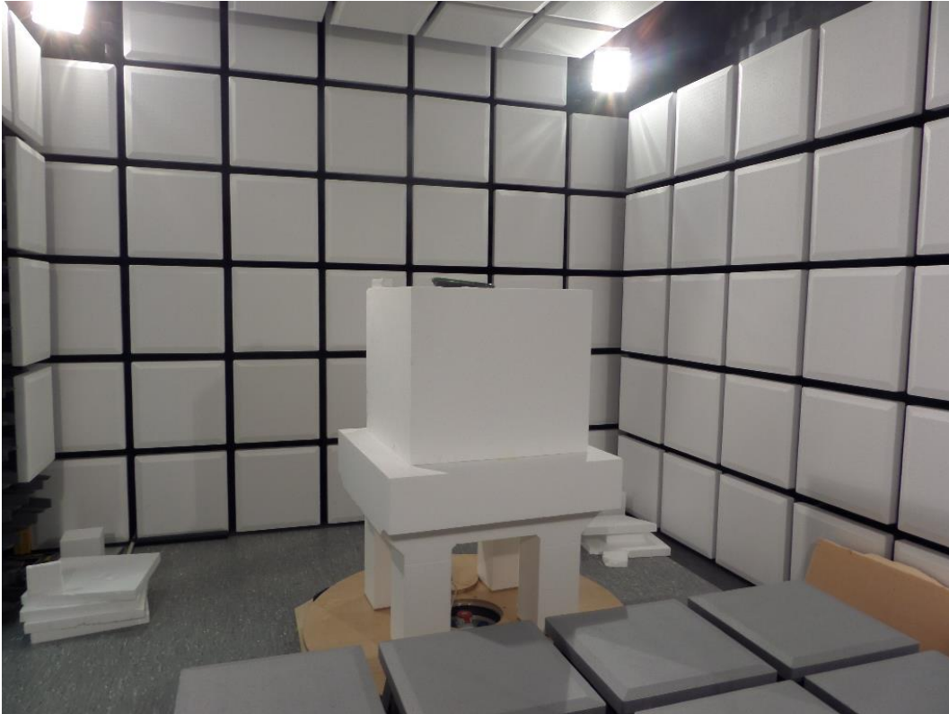
Anechoic room – Position 2 supplied by battery
