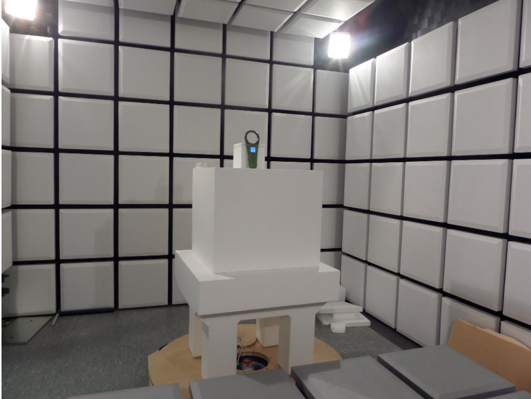
Anechoic room – Position 1 supplied by battery
