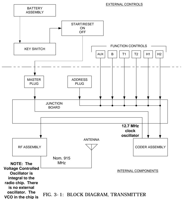
FIG. 3-1: BLOCK DIAGRAM, TRANSMITTER
