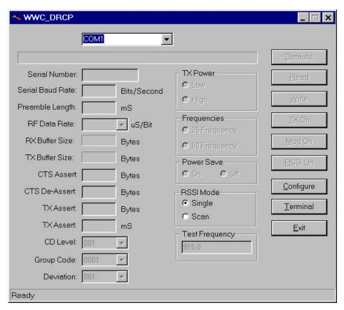
2. Select the appropriate COM port to which the radio is connected.
