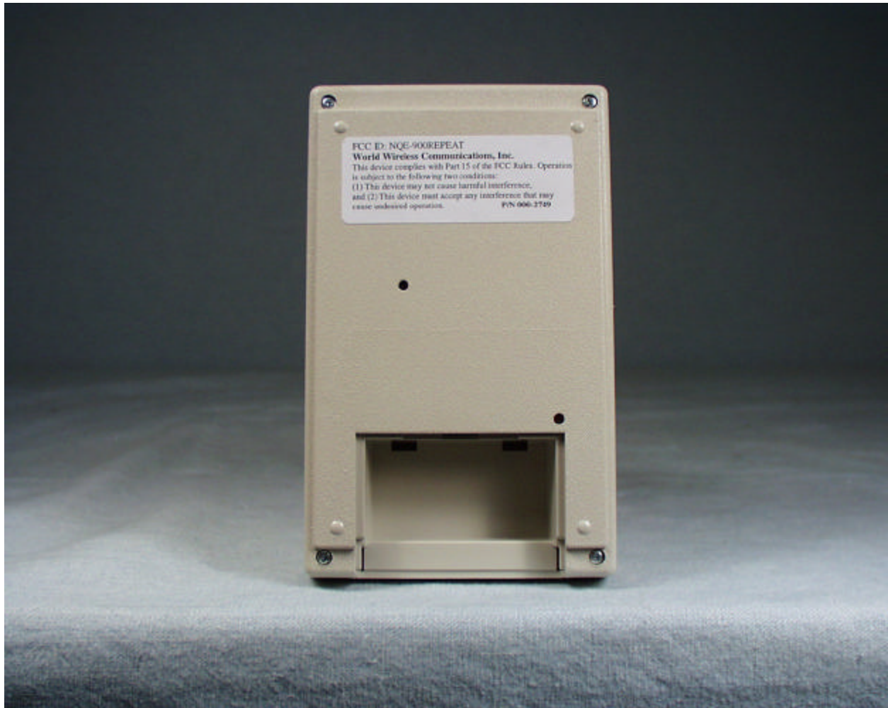
Back View of the 900 REPEATER with battery cover removed
