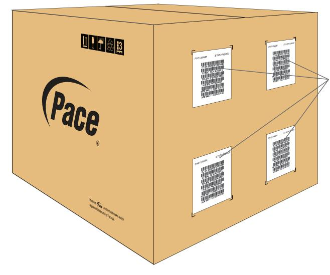
Position 4 x CARTON label **E118-PX013ANM-Carton-Label-RevA** (one per unit) as squarely as possible between the corner tick marks in positions shown.
