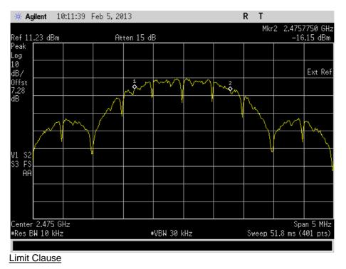
The minimum 6 dB Bandwidth shall be at least 500 kHz.
