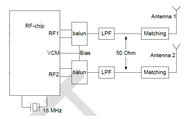
Each path is used as TX or RX path. Only one path per time is used.
