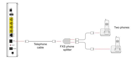
After your gateway recognizes the phones (Line 1 and Line 2), the **VOICE 1** and **VOICE 2** indicators turn steady green and blink when the associated phone is active.
