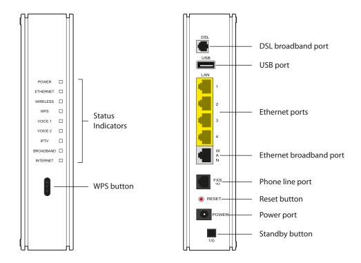
Use WPS (Wi-Fi Protected Setup) to simplify the process of connecting wireless devices to the network. For more information, go to your gateway configuration page at http://192.168.1.254
