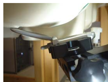
Figure 14.7 Right Head SAR Test Setup -- Ear / 15° Tilt Position --
