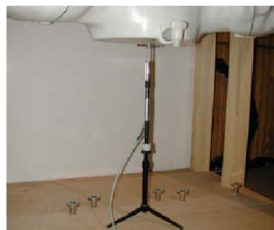
Figure 12.1 Dipole Validation Test Setup
