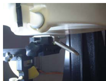
Figure 14.5 Body SAR Test Setup -- Body Position --
