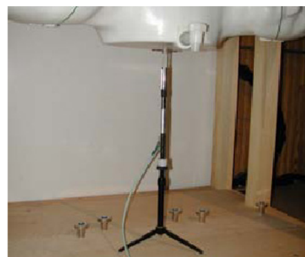
Figure 12.1 Dipole Validation Test Setup
