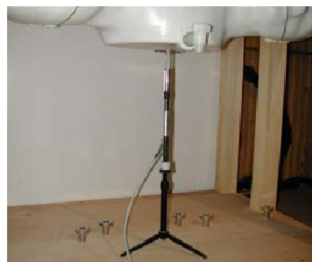
Figure 12.1 Dipole Validation Test Setup
