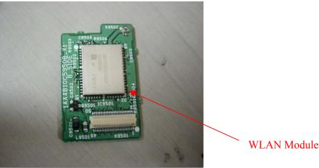
Fig 2. Front view of "QXXAVC922---P" to be equipped for a projector (example)
