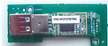
The board installed this modular transmitter
