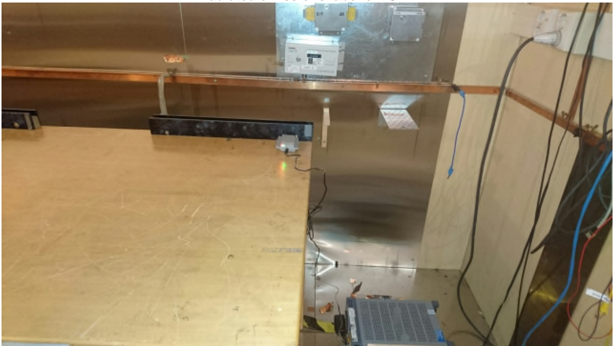
Power line conducted emission during charging of the battery
