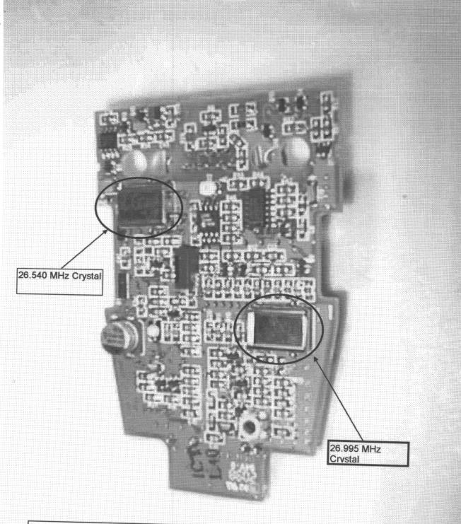
FCCID NPI71846 Tower Unit Model 71846 Printed Circuit Board Component Side
