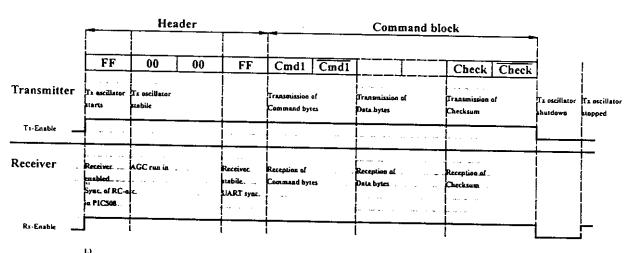
The first Headerbyte, from PC to Tower Unit, is also used for syncronisation of the internal RC-oscillator inside the PIC508 microcontroller Because of this, is the first byte, from the PC to Tower Unit, not FF, but FE instead.
