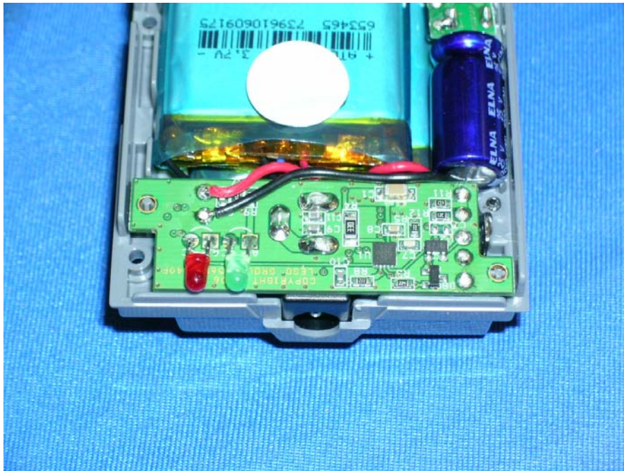
Rechargeable Battery Pack PCB solder side
