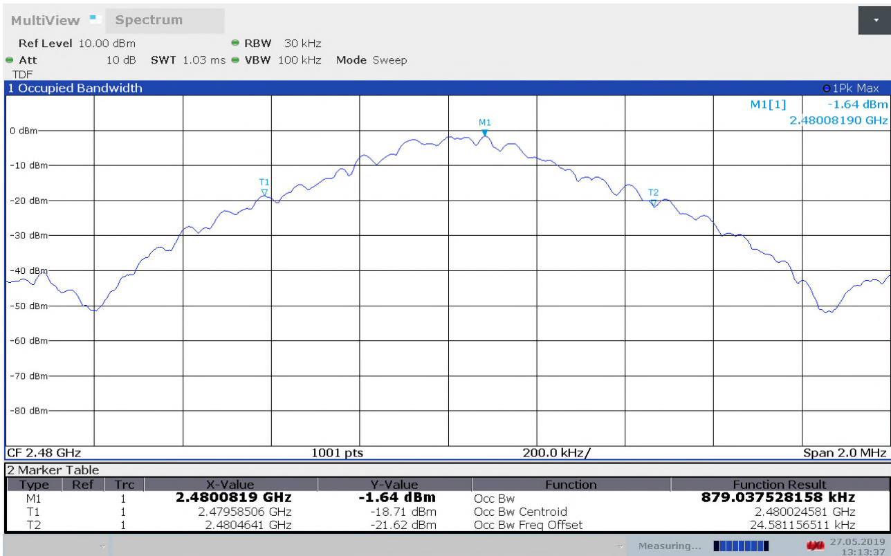
99% Bandwidth – GFSK, ch2480MHz
