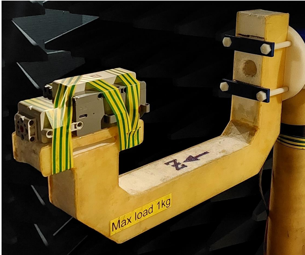
Figure 3: Placement of AUT on turn arm in chamber showing Z-axis
