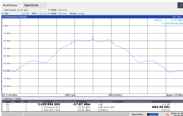
DTS BW, 2440 MHz, 1M
