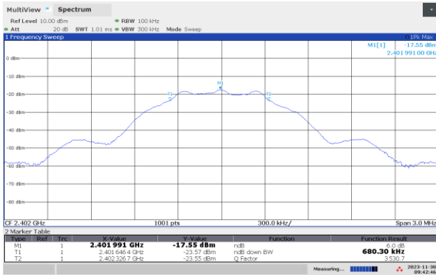
DTS BW, 2402 MHz, 1M
