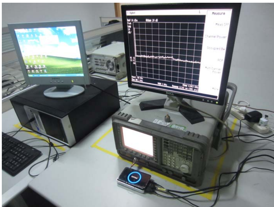
SPURIOUS EMISSION TEST SETUP
