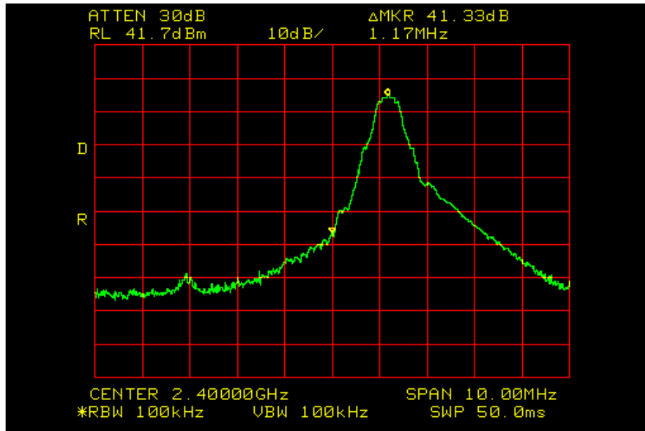
Bandedge Spurious – 15.247(c) – EUT set for Maximum data modulated output power, Channel 1
