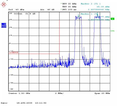
Intermodulation Characteristics 20 Watts per carrier / 40 Watts composite
