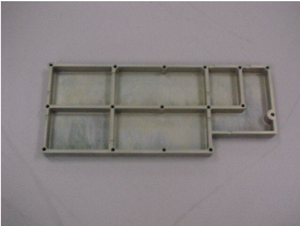
G16: 3 ST EMI CONTAINMENT (INSIDE VIEW)
