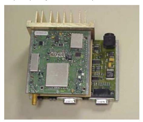
2. Bottom assembly, showing top of RF Board and bottom of Modem.
