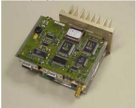
3. Exploded view: showing top of modem, top of RF Board, and separating plate.
