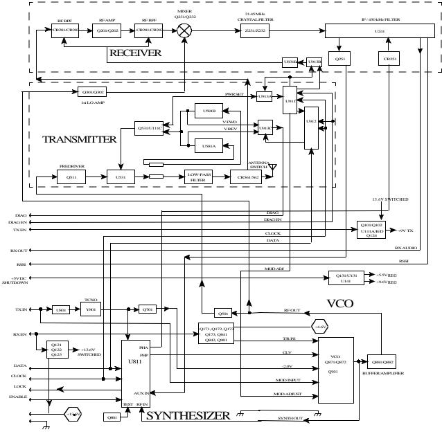
Figure 4-2 Transceiver Block Diagram
