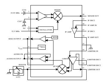
Figure 4-3 U241 Block Diagram
