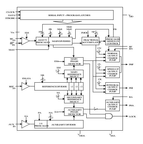
Figure 4-1 U811 Synthesizer Block Diagram
