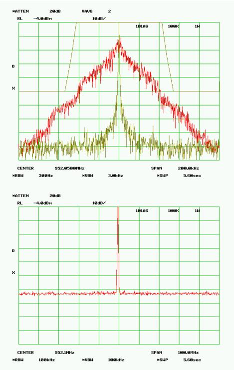
MASK 101.111a6 100 kHz- 10 Watts RF Frequency 952.050 MHz SPECTRUM FOR EMISSION - 51K3F1D Data Rate = 256kbps PEAK DEVIATION = 13.77 kHz
