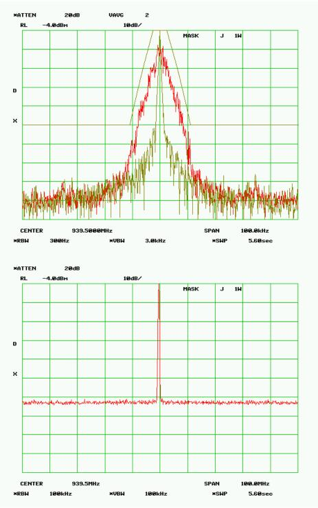
MASK J – 10.0 Watts RF Frequency 939.500 MHz SPECTRUM FOR EMISSION - 8K08F1D Data Rate = 32 kbps PEAK DEVIATION = 3.728 kHz
