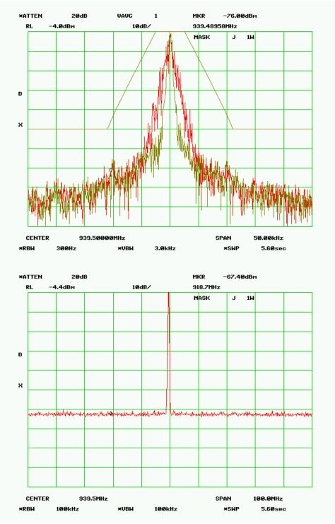
MASK J – 10.0 Watts RF Frequency 939.500 MHz SPECTRUM FOR EMISSION - 3K55F1D Data Rate = 8 kbps PEAK DEVIATION = 1.09 kHz
