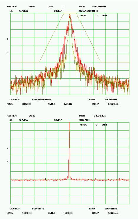
MASK J – 1.0 Watts RF Frequency 939.500 MHz SPECTRUM FOR EMISSION - 3K20F1D Data Rate = 12 kbps PEAK DEVIATION = 1.15 kHz
