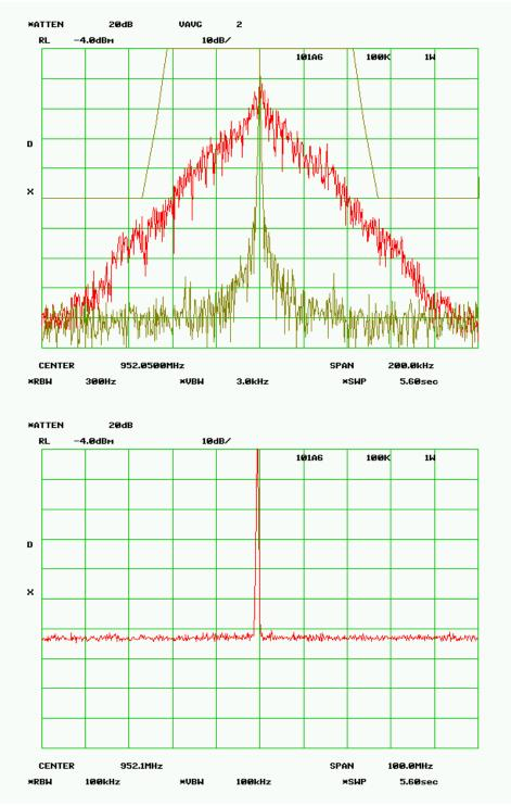
MASK 101.111a6 100 kHz- 10 Watts RF Frequency 952.050 MHz SPECTRUM FOR EMISSION - 49K7F1D Data Rate = 192kbps PEAK DEVIATION = 13.02 kHz
