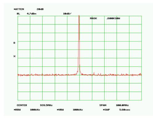
MASK J - 100 kHz - 1.0 Watts RF Frequency 939.500 MHz SPECTRUM FOR EMISSION - 49K7F1D Data Rate = 192 kbps PEAK DEVIATION = 13.02 kHz
