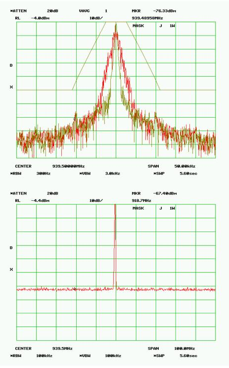
MASK J – 10.0 Watts RF Frequency 939.500 MHz SPECTRUM FOR EMISSION - 3K20F1D Data Rate = 12 kbps PEAK DEVIATION = 1.15 kHz
