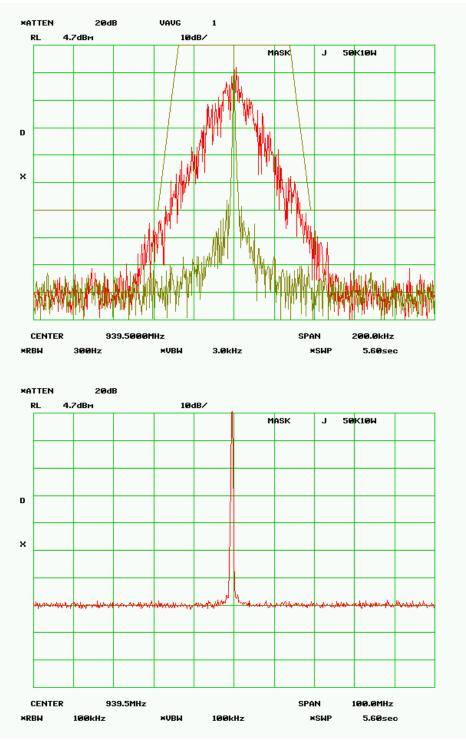
12.0 Mask J – Part 90.210(j) Aggregation for 100 kHz Channel
