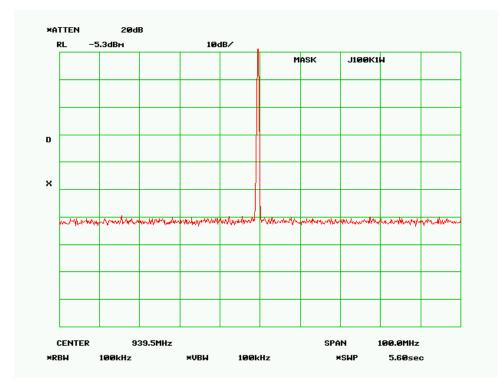
MASK J - 100 kHz - 10.0 Watts RF Frequency 939.500 MHz SPECTRUM FOR EMISSION - 49K7F1D Data Rate = 192 kbps PEAK DEVIATION = 13.02 kHz
