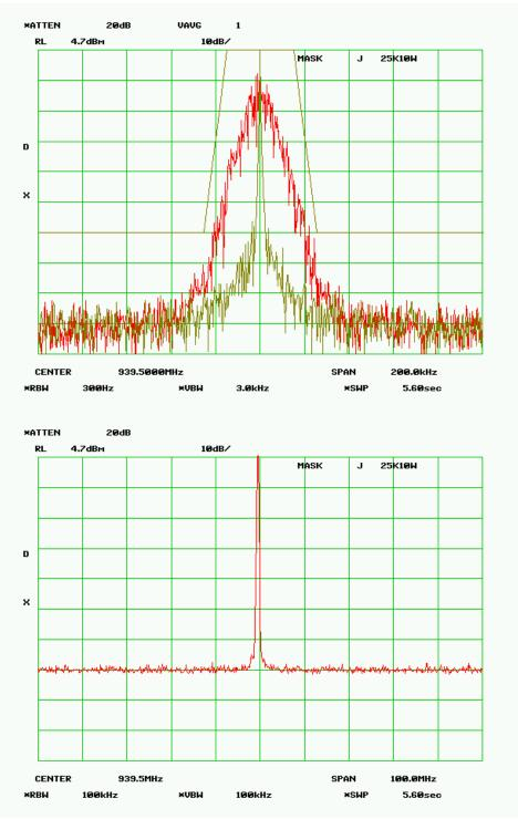
11.0 Mask J – Part 90.210(j) Aggregation for 50 kHz Channel
