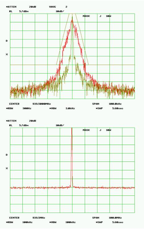
MASK J – 1.0 Watts RF Frequency 939.500 MHz SPECTRUM FOR EMISSION - 8K50F1D Data Rate = 24 kbps PEAK DEVIATION = 3.725 kHz
