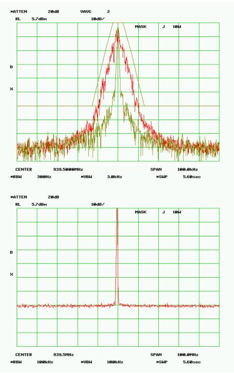
10.0 Mask J – Part 90.210(j) Aggregation for 25 kHz Channel
