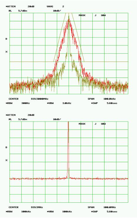
MASK J – 1.0 Watts RF Frequency 939.500 MHz SPECTRUM FOR EMISSION - 8K08F1D Data Rate = 32 kbps PEAK DEVIATION = 3.728 kHz
