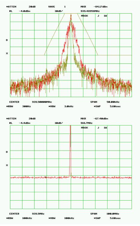
MASK J – 10.0 Watts RF Frequency 939.500 MHz SPECTRUM FOR EMISSION - 3K30F1D Data Rate = 4 kbps PEAK DEVIATION = 1.15 kHz
