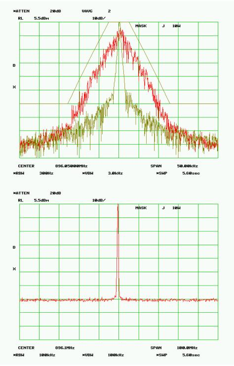
MASK J - 1.0 Watt RF Frequency 896.050 MHz SPECTRUM FOR EMISSION - 8K08F1D Data Rate = 32 kbps PEAK DEVIATION = 3.728 kHz
