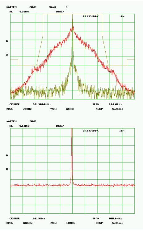
MASK 24.133a1 - 100 kHz - 1.0 Watts RF Frequency 901.900 SPECTRUM FOR EMISSION - 51K3F1D Data Rate = 256kbps PEAK DEVIATION = 13.77 kHz
