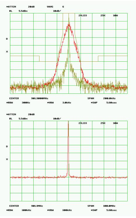
MASK 24.133a1 - 25 kHz - 1.0 Watts RF Frequency 901.900 SPECTRUM FOR EMISSION - 17K8F1D Data Rate = 48 kbps PEAK DEVIATION = 7.59 kHz
