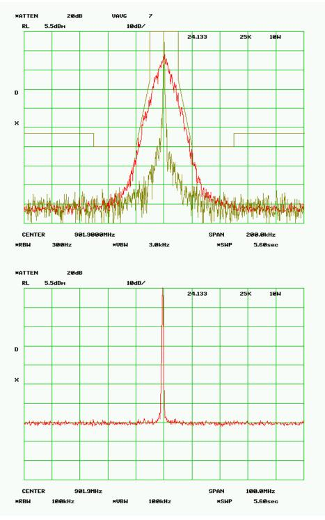
MASK 24.133a1 - 25 kHz - 1.0 Watts RF Frequency 901.900 SPECTRUM FOR EMISSION - 17K0F1D Data Rate = 64 kbps PEAK DEVIATION = 7.52 kHz
