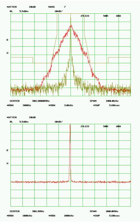
MASK 24.133a1 - 50 kHz - 1.0 Watts RF Frequency 901.900 SPECTRUM FOR EMISSION - 30K0F1D Data Rate = 64 kbps PEAK DEVIATION = 11.02 kHz
