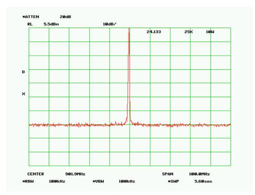
MASK 24.133a1 - 25 kHz - 1.0 Watts RF Frequency 901.900 SPECTRUM FOR EMISSION - 16K8F1D Data Rate = 32 kbps PEAK DEVIATION = 6.30 kHz
