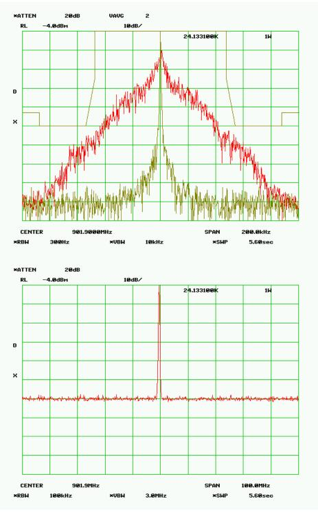
MASK 24.133a1 - 100 kHz - 10.0 Watts RF Frequency 901.900 MHz SPECTRUM FOR EMISSION - 51K3F1D Data Rate = 256kbps PEAK DEVIATION = 13.77 kHz
