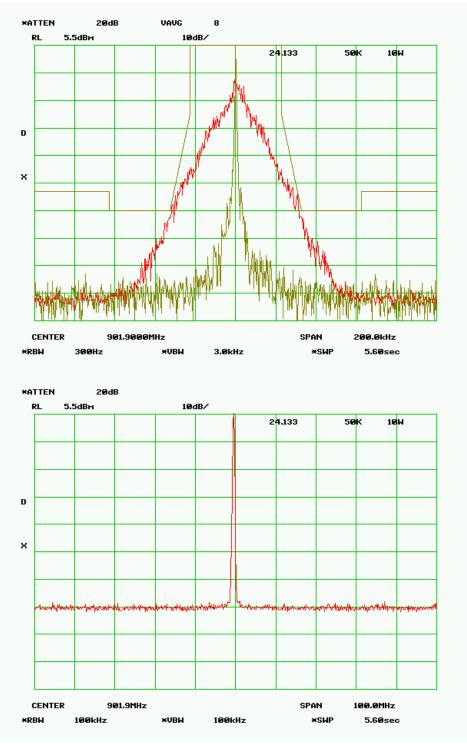
MASK 24.133a1 - 50 kHz - 1.0 Watts RF Frequency 901.900 SPECTRUM FOR EMISSION - 29K5F1D Data Rate = 96 kbps PEAK DEVIATION = 10.81 kHz
