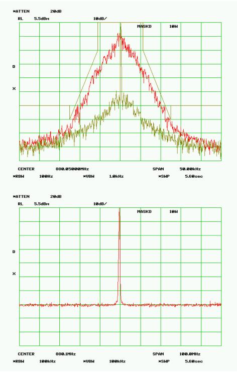
MASK D - 1.0 Watt RF Frequency 880.050 MHz SPECTRUM FOR EMISSION - 8K08F1D Data Rate = 32 kbps PEAK DEVIATION = 3.728 kHz
