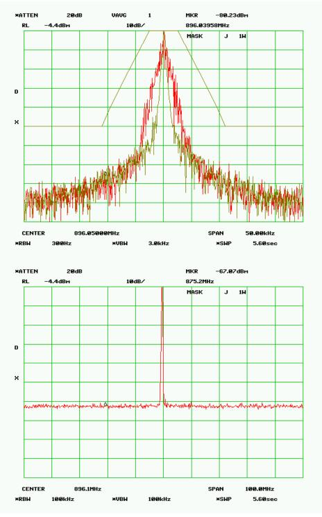
MASK J – 10.0 Watts RF Frequency 896.050 MHz SPECTRUM FOR EMISSION - 3K20F1D Data Rate = 12 kbps PEAK DEVIATION = 1.15 kHz
