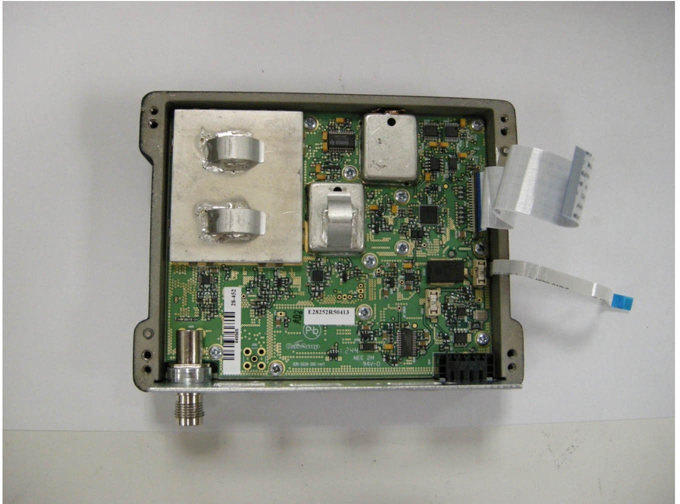
RF Board Metal Plate Removed
