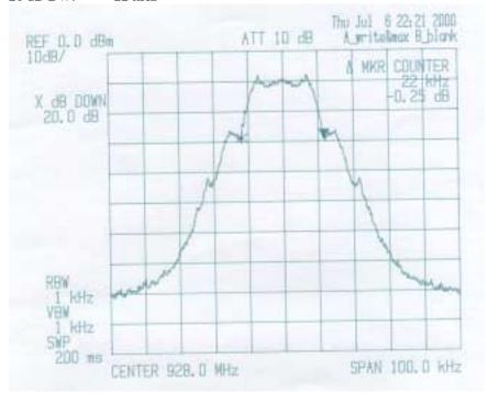
FCC Part 15.247, Frequency Hopping Wireless Modem
