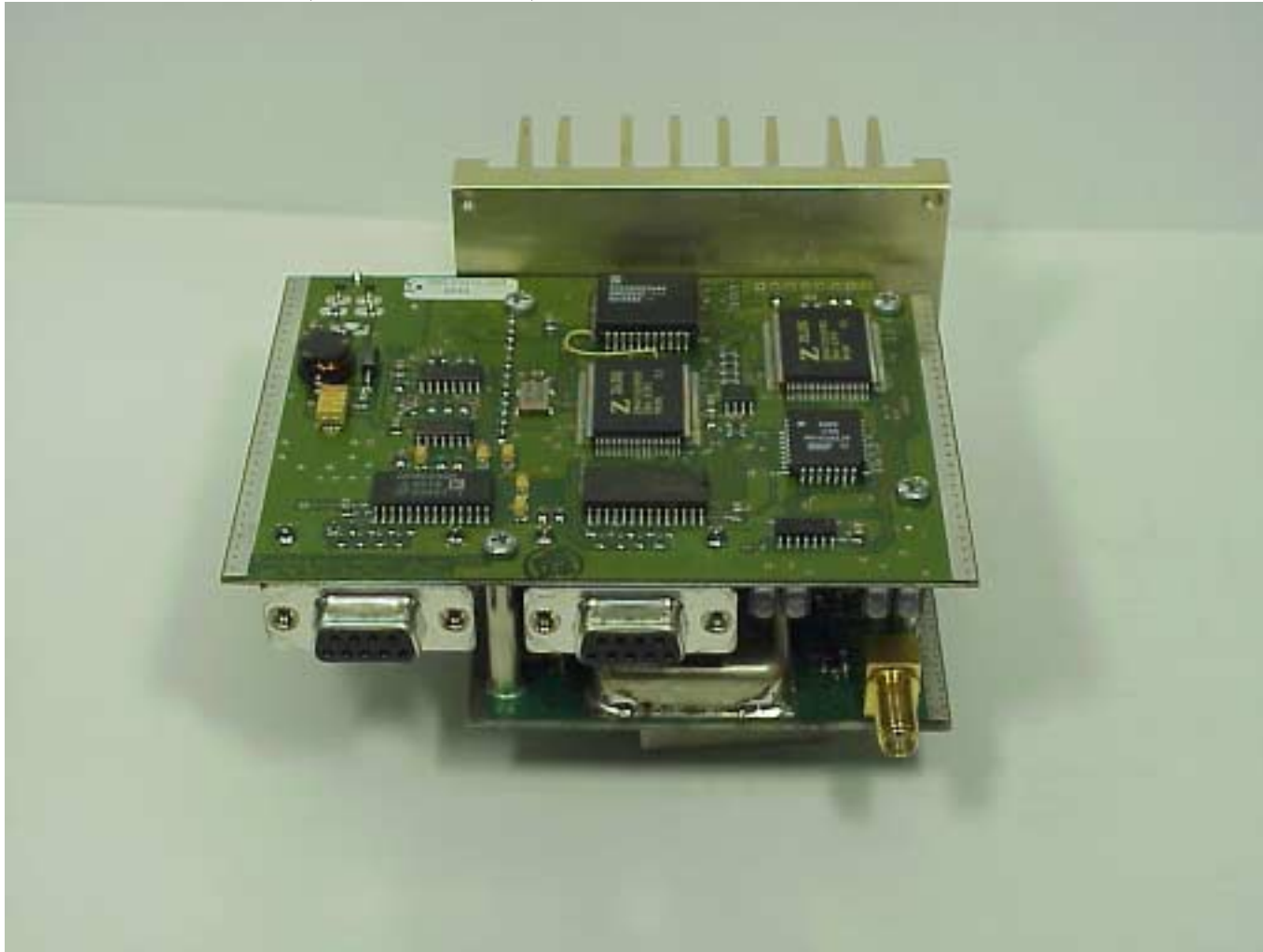
Photo 3: Internal (RF and Modem)
