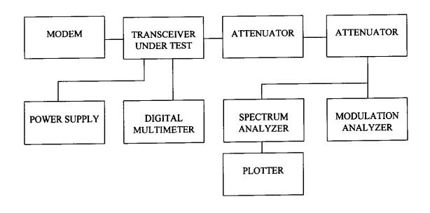
Transmitter Occupied Bandwidth (Continued) DL-3286 Modem at 4800 BAUD (9600 bps) In Support of Emission Designator 13K0F1D
