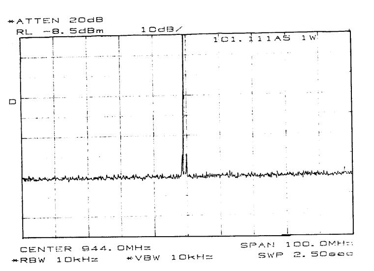
NAME OF TEST: Transmitter Occupied Bandwidth
