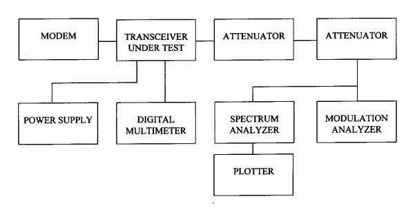
Transmitter Occupied Bandwidth (Continued) DL-3286 Modem at 4800 BAUD (9600 bps) In Support of Emission Designator 16K0F1D
