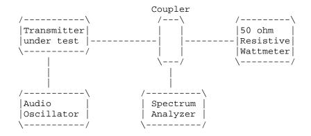
Spurious\_emissions\_at\_antenna\_terminals(conducted): Data on the following page shows the level of conducted spurious responses. The carrier was modulated 100% using a 2500Hz tone. The spectrum was scanned from 0.4 to at least the 10th harmonic of the fundamental. The measurements were made in accordance with standard TIA/EIA-603.
