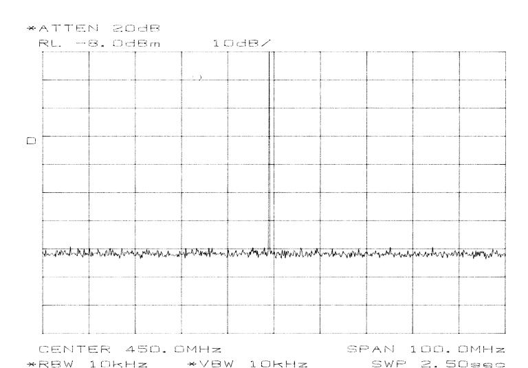
NAME OF TEST: Transmitter Occupied Bandwidth
