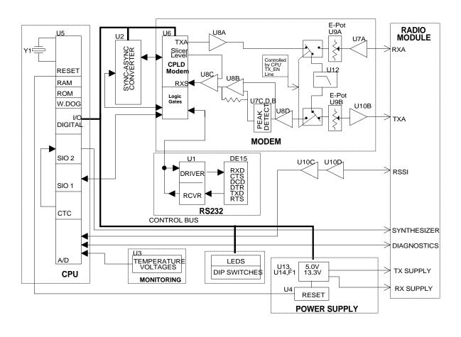
Figure 3: HNET MODEM BLOCK DIAGRAM
