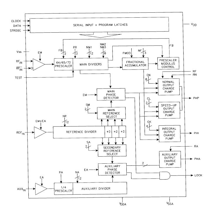
Figure 1: DL-3422 SYNTHESIZER INTEGRATED CIRCUIT (U811)
