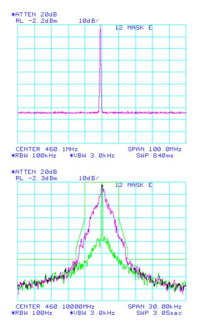
Mask: E, 1W Output Power = 1 Watt Spectrum for Emission:3K45 F1DData Rate:16 kbpsPeak Deviation with Data:1.056 kHz
