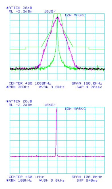
Mask: C, 1W Output Power = 1 Watt Spectrum for Emission:17K0 F1DData Rate:64 kbpsPeak Deviation with Data:7.52 kHz
