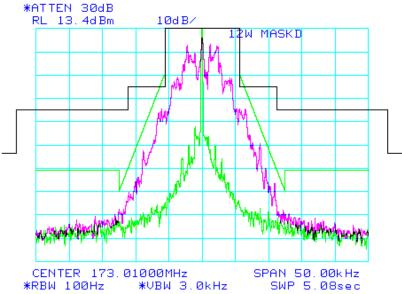
Mask: D, 1W Output Power = 1 Watt Spectrum for Emission: 10K2F3E
