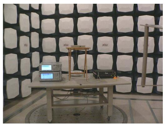
14.4 Radiated Spurious Emissions - Rear View (TX Mode)
