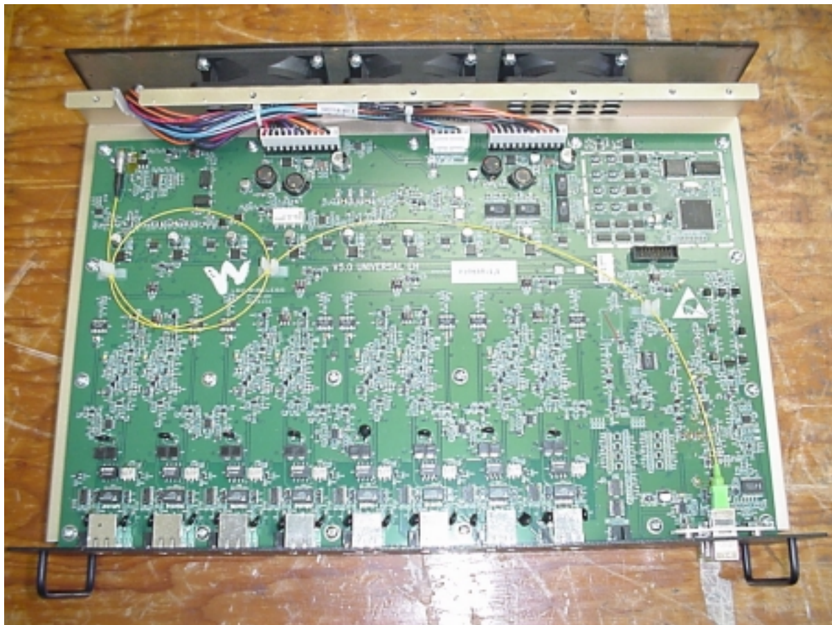
INSIDE OF EXPANSION HUB
