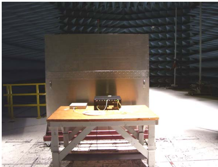
Photograph 2. Conducted Emissions Test Setup, Front View
