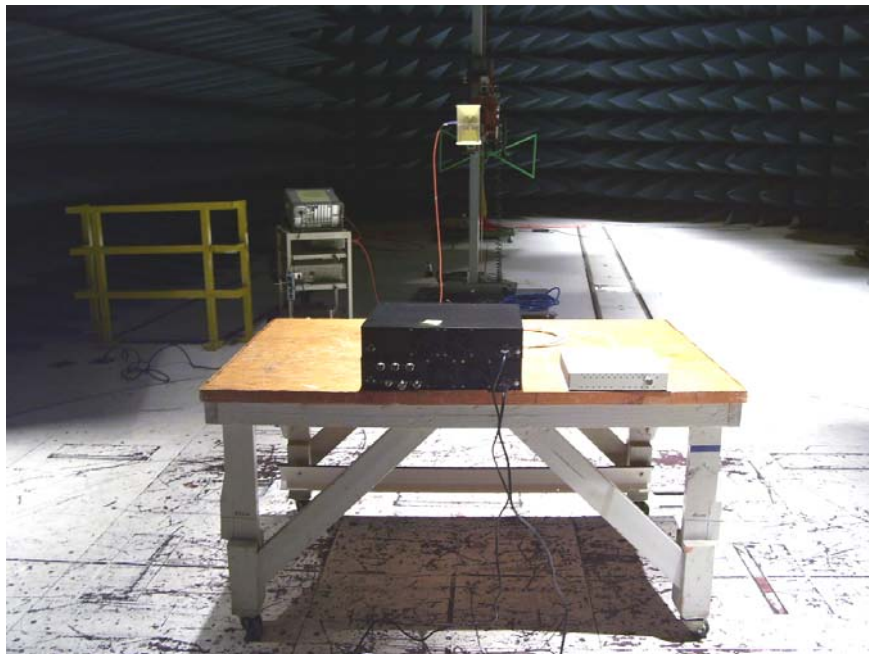
Photograph 7. Radiated Emission Limits Test Setup, 1 GHz to 10 GHz, Back View
